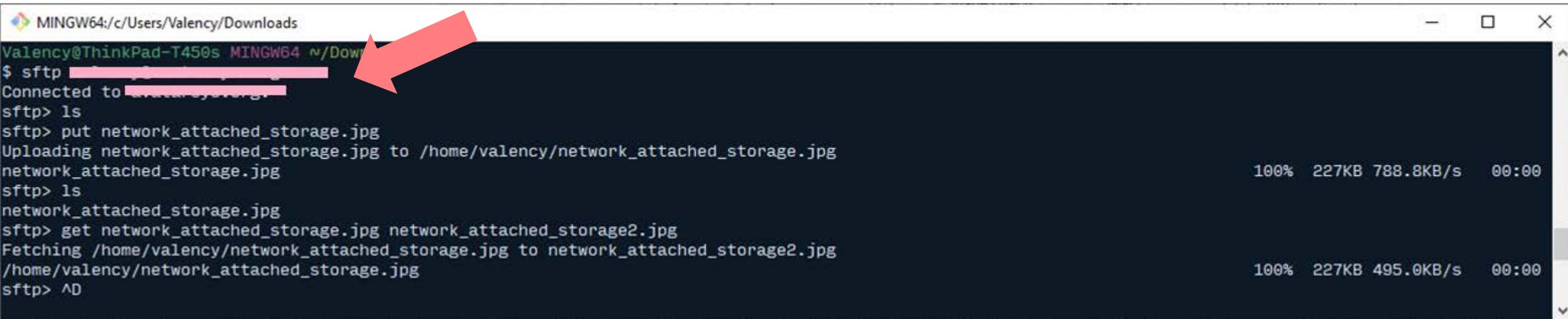
A terminal window showing an SFTP session. The prompt is \$ sftp [redacted]. The user connects to [redacted]. They list files (ls), upload network\_attached\_storage.jpg, and then download it to network\_attached\_storage2.jpg. A red arrow points to the redacted IP address in the sftp command.
