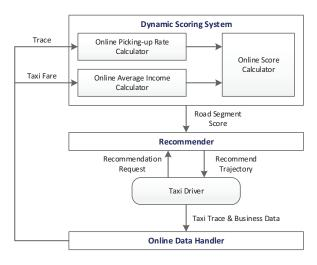
Fig. 5. System structure of HUNTS.
