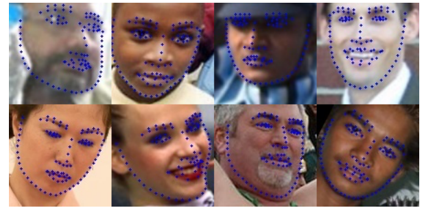
Figure 1. Landmarks inferred by PLA where the dots represent predicted landmarks. PLA is capable of handling head deflection and partially occluded images.
